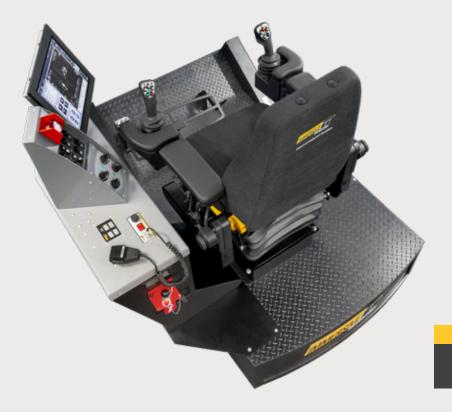
High Fidelity LCD Operator Interface - Centurion 6 System with Adaptive Controls and Pay Load 2.
