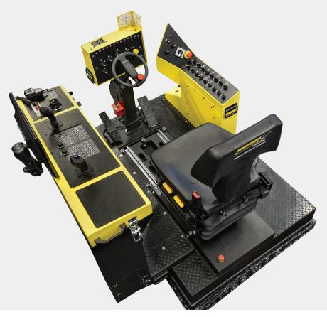
Epiroc Rig Control System (RCS 5) with 15 inch touch screen and multi-function joysticks enable drill and hyraulic control proficiency training.
