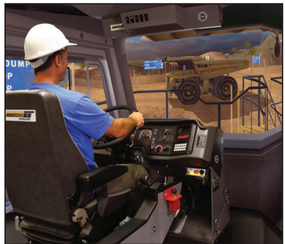
Immersive Technologies' Advanced Equipment Simulator with a Caterpillar Haul Truck Conversion Kit® installed.
