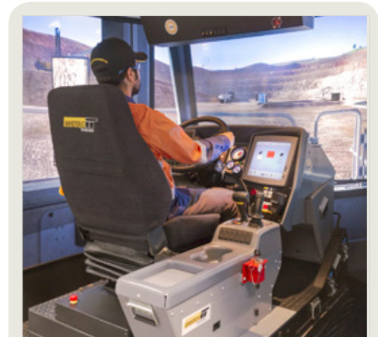
Operator training using Immersive Technologies' Advanced Equipment Simulators reduced haul truck fuel consumption by 6.9% in five months.
