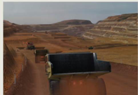
Through simulation operators are trained to identify and correct errors such as brake misuse to optimize tire life.
